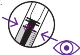
5. Slowly, drop-by-drop, add reagent MG-3 while swirling (important!). Continue adding reagent MG-3 drop-wise until the solution turns completely grey or blue. The grey or blue colour must still be present after 30 seconds, if not continue adding MG-3 until the water finally turns grey or blue.
